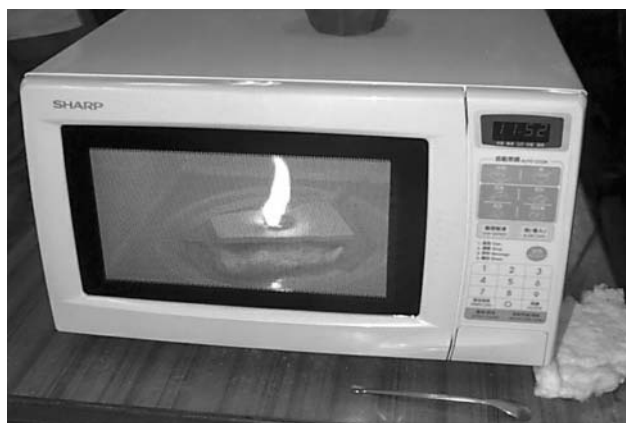
Fig. 1 Glow typically observed inside the microwave oven during the reaction between \text{Li}_2\text{CO}_3 and \text{Co}_3\text{O}_4 .
